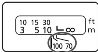
The infrared index corrects the focus setting when using monochrome infrared film. Focus on the subject manually, then adjust the distance setting by moving the focusing ring to the corresponding infrared index mark.
